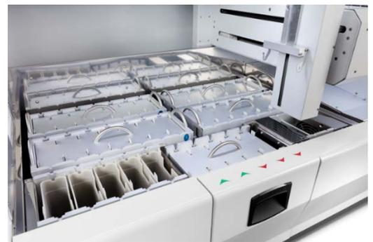
The agitation of the reagent dishes is particular and innovative, it is completely independent from the automatic arm. This particular agitation system (called "WAVING") allows to obtain homogeneity of the staining solution inside the dish, improving the quality of section staining and, last but not least, it reduces the amount of precipitate produced during daily routine.
