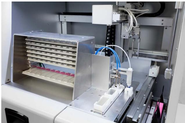
Unique and exclusive exit system of mounted glass slides: Bio-optica instrument ALLOWS TO OBTAIN THE MOUNTED GLASS SLIDES DIRECTLY ON TRAYS IN HORIZONTAL POSITION, by avoiding a huge time waste for the operators who will be able to bring the trays directly to the pathologist for the evaluation at the microscope.
